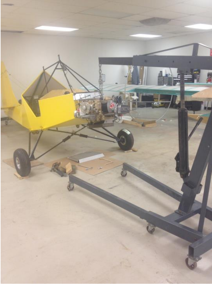
Tom Jeschke's Double Eagle. The engine getting ready to be hung. Bob Vandenberg came through with finishing tape that was requested earlier in January .
